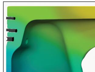
Piston with TAC ring groove geometry (cold engine)
