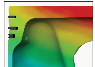
Piston with TAC ring groove geometry (at operating temp)
