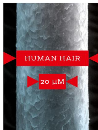
[FIG.20] Comparison between a human hair and the minimum permitted clearance of a con rod bearing of 20 μm.
