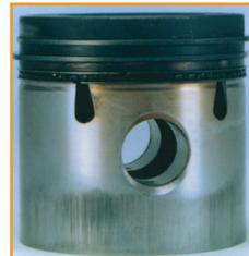
**Symptom:** Engine does not develop normal full power. Engine may overheat.
