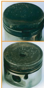
**Symptom:** Engine noise: Pinging/loss of power.
