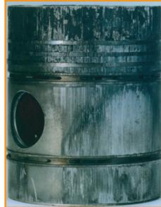
**Symptom:** Loss of power. Engine noise. Fumes from the engine breather.
