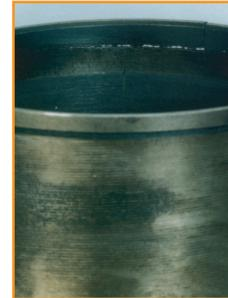
**Symptom:** Combustion gases ventilating to coolant, Engine noise, Eventual destruction of liner.
