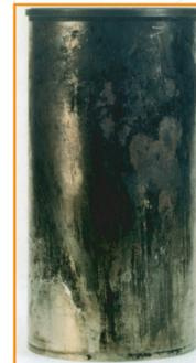
**Symptom:** Loss of power. Oil consumption. Fumes from engine breather. Piston seizure in extreme cases.
