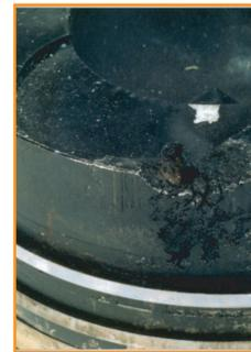
**Symptom:** Loss of power, emission of fumes from engine breather. Exhaust smoke.
