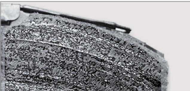
**APPEARANCE** Contaminated pad friction material.
