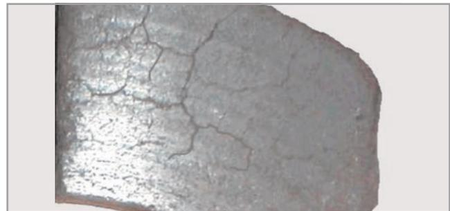
**APPEARANCE** Pad with surface cracks.
