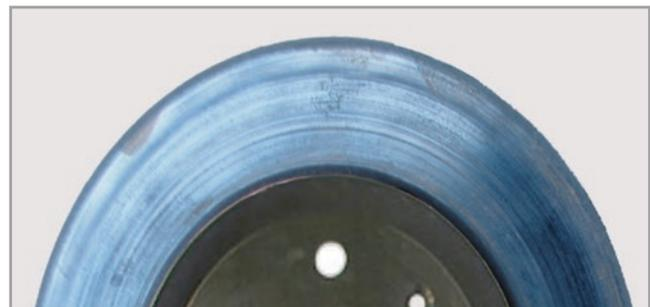
**APPEARANCE** Blue stripes on the rotor indicating a physical change due to overheating.
