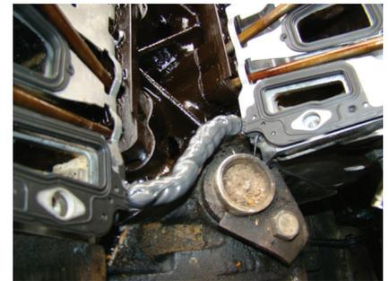
PermaDryPlus® intake gaskets installed dry:
