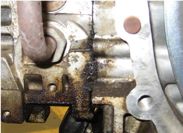
External oil leak from failed head gasket
