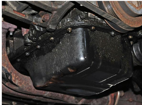
Leaking OE oil pan gasket
