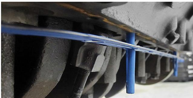
Fel-Pro has developed an innovative and easy solution to these issues. Fel-Pro oil pan SnapUps are the clean, simple and effective way to speed up an oil pan gasket replacement. Simply thread them into the block where the oil pan bolts go, snap the oil pan gasket in place, followed by the pan itself, and start threading the bolts in. Once the oil pan is secure, the SnapUps are easily removed and are reusable.
