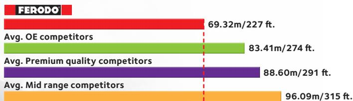
Water was sprayed directly on to the brake disc, as well as on to the road surface, to create the most realistic and consistent wet conditions for every brake setup. Each product was tested with 6 brake applications from 80 km/h to 0 km/h (50 to 0 mph).
