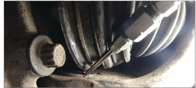
*In applications with tight clearances, low-profile zerk make injecting fresh grease easy and possible.*
