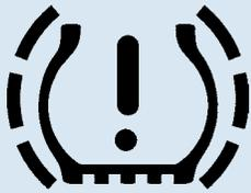
This system monitors the air pressure in the tires with a wheel-mounted sensor. The direct type of TPMS can detect actual pressure levels and transmit the information to the driver more quickly. Tires are monitored individually by sensors attached to a special tire valve or strapped to the drop center of each wheel. Each sensor monitors and transmits tire pressure to the ECU. On some models, the temperature is also monitored to compensate for cold and warm pressure variations.
