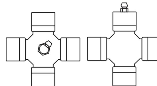
**Part No. U-Joint Grease Fitting**
