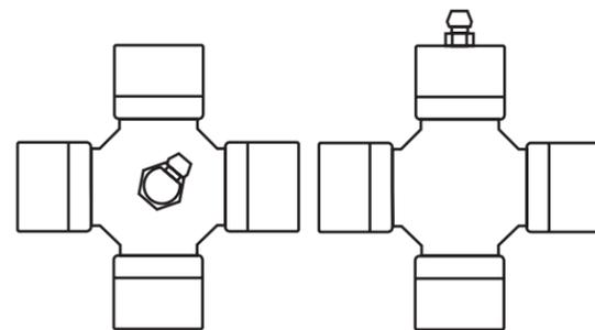
**Part No. U-Joint Grease Fitting**
