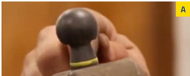
Ball joint stud in an undamaged steering knuckle.
