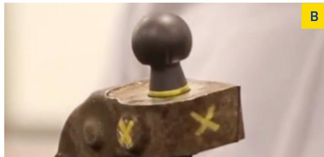
Ball joint stud in a damaged steering knuckle.
