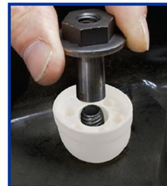
Easier to install than traditional sway bar link kits, the MOOG Problem Solver bolt style sway bar link features patented molded bushings that center and hold the coated washers in place, making them easier to install. Instead of a standard nut, MOOG sway bar link kits use a 1"-barrel lock nut that can easily be threaded on, even if the bolt end is flush with the washer. This saves time during installation.
