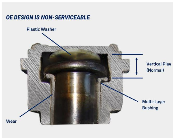
Premature slider (or telescoping) ball joint failures are a common occurrence on many late-model Dodge and RAM trucks and Jeep SUVs equipped with a straight or solid axle. The OE ball joints are not greaseable, which can increase the rate at which they wear. As the ball joint wears, looseness develops in the socket. Vertical movement of the stud is normal, but once radial movement (side-to-side or back-and-forth play) exceeds manufacturer specifications, it's time to replace the ball joint.
