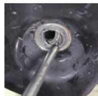
**Technician can easily align the bushing sleeve to the bolt hole.**
