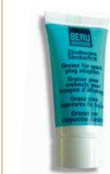
In order to ensure that the transmission of high voltage is safe and reliable, the plug-shaft ignition coils are very firmly attached to the spark plugs. Due to the resulting high temperatures, there is a risk of the spark plug fusing with the ignition coils' silicone plug. It is therefore essential that BERU plug grease (order no. 0 890 300 029 with 10g or 0 890 300 045 with 50g) is used when a spark plug is changed. This ensures that plugs are also easily removed.
