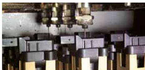
The secondary wire is embedded in the casting resin by vacuum casting.
