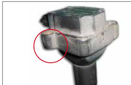
Crack formation on the ignition coil insulation due to strain during installation.
