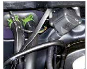
Ignition coils that are directly mounted on the bulkhead are especially exposed. The possible consequence is oxidation of the contacts.
