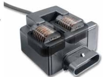
In comparison with conventional coils, the new ignition technology from BERU offers a significantly shorter ignition lag and better combustion stability over the entire combustion cycle; especially, however, in the partial load range and when idling. The integrated electronics enables seamlessly sequential charging and discharging of the coils as well as variable adjustment of the ignition energy. The advantage is minimum energy consumption over the entire running cycle.
