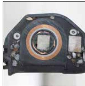
**Copy:** Ignition coil housing and high-voltage cable have been filled with gravel to save on expensive casting compound. Air bubbles have formed in the gaps, the impregnation quality suffers, especially in the high-voltage section: If air collects in the secondary winding, it will become ionized – this means the air becomes conductive and in effect corrodes the coil housing until a ground potential is reached. This will result in a short circuit or flash-over and failure of the ignition coil.
