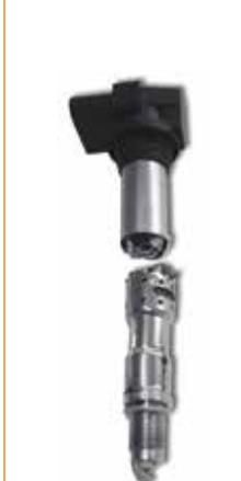
Only the spark plug was to be exchanged. Because of the wrong removal tool, now the coil has to be replaced as well.
