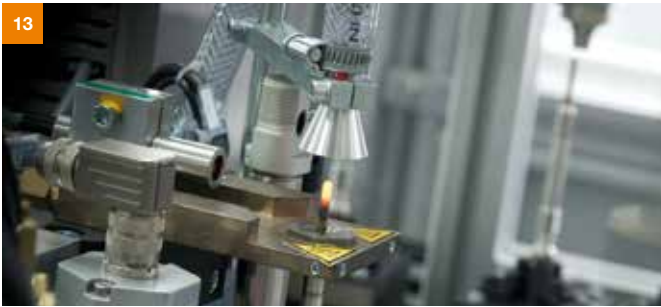
100% functional testing of the PSG: The glow test proves that the plug reaches the required temperature in the allotted time.
