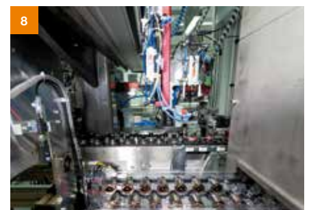
The glow current connector is fed through the duct inside the sensor module.
