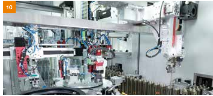
In the logistics module, the parts are moved from the first to the second production train, where pre-assembly of the end cap initially takes place.
