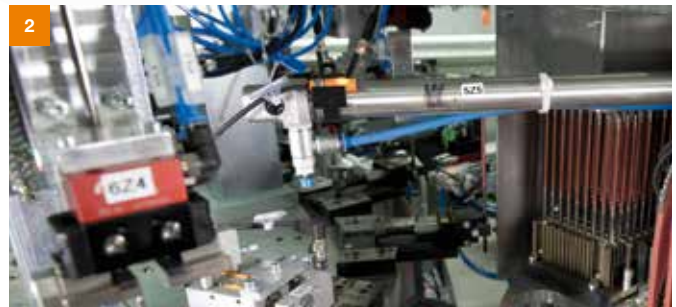
Start of the fully automated production process: The installation of the heating element and its extension...
