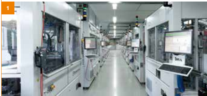
A look at the modular production line for PSG pressure sensor glow plugs.
