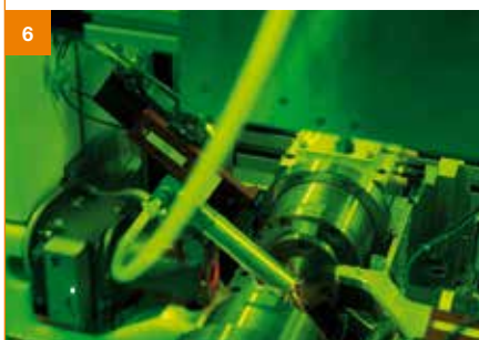
Then the glow power connector is mounted and welded on the inner terminal.
