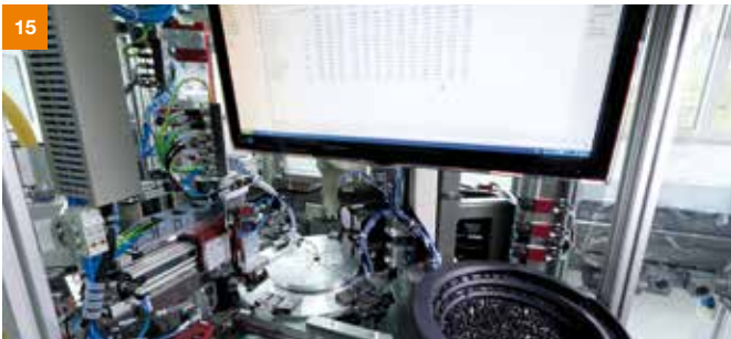
This is now followed by geometry testing of the plug: The final dimensions and precise concentricity are documented by a camera system.
