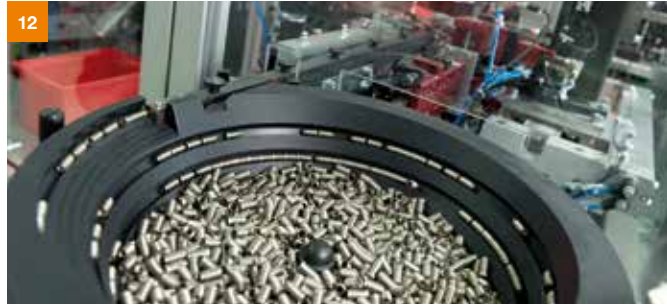
To achieve flexible bearing of the heating rod, the glow tube is surrounded by a boot. The figure shows the boot feeding via a conveyor rail.
