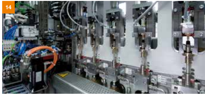
Then leak testing is performed.
