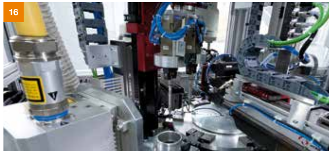
Only plugs that have passed all the tests, are transported on to the next step, laser marking.
