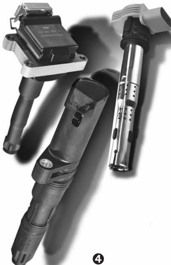
Various designs of plug shaft/connector ignition coils for new vehicle models BMW, Fiat, Mercedes-Benz, Porsche, Renault or VW.
