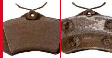
**Appearance.** Rust between the friction material and back plate.
