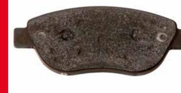
**Appearance.** The friction material is totally worn out.
