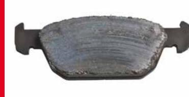
**Appearance.** The brake pad friction material is glazed
