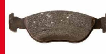
**Appearance.** Metal ingrained on the friction surface.
