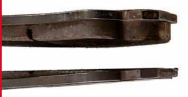
**Appearance.** One or more brake pads within an axle set is extremely worn.
