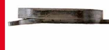
**Appearance.** A back plate that is damaged.
