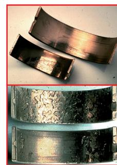
**Symptom:** Breakouts of lining material showing „bark-beetle“ pattern in main loaded zone of bearing.
