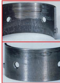
**Symptom:** Localised surface disruption of bearing surface. The back of the bearing will be marked or indented behind the area of damage.
