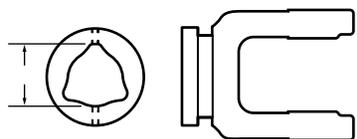
Inner Tube Yoke – Part No. 1042
