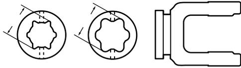
Inner Tube Yoke – **Part No. 1647**
