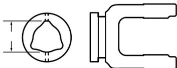
Inner Tube Yoke – **Part No. 1049**
