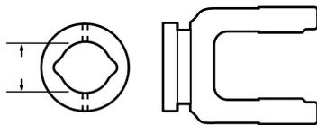
Inner Tube Yoke – Part No. 1642
