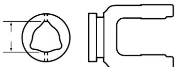
Inner Tube Yoke – **Part No. 1047**
