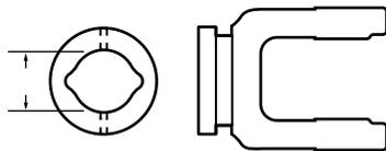
Inner Tube Yoke – **Part No. 1646**
