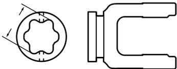
Inner Tube Yoke – **Part No. 1648**
