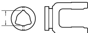
Inner Tube Yoke – Part No. 1043
