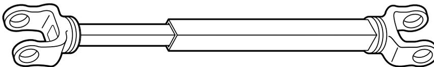
Telescoping Drive Shaft Assembly – **Part No. 1248**
