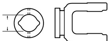
Inner Tube Yoke – **Part No. 1643**
