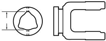
Inner Tube Yoke – **Part No. 1048**
