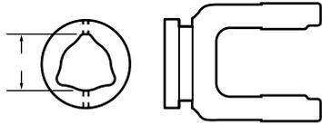
Inner Tube Yoke – **Part No. 1044**
