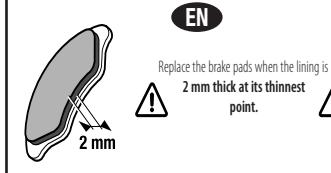
EN Replace the brake pads when the lining is 2 mm thick at its thinnest point.
