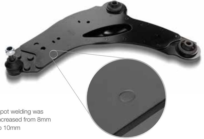
Spot welding was increased from 8mm to 10mm
