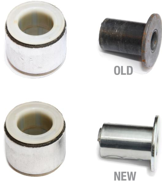
A smooth chromium-based coating and additional grease between the metallic and plastic part reduces friction and prevents noise when the parts move.
