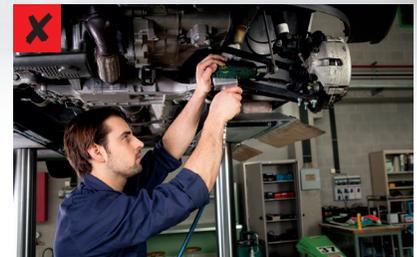
Don't use a torque gun: you risk damaging and/or a reduced performance of the parts.
