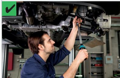
Do use a torque wrench such as a dynamometric key for the correct method for fixing the part.
